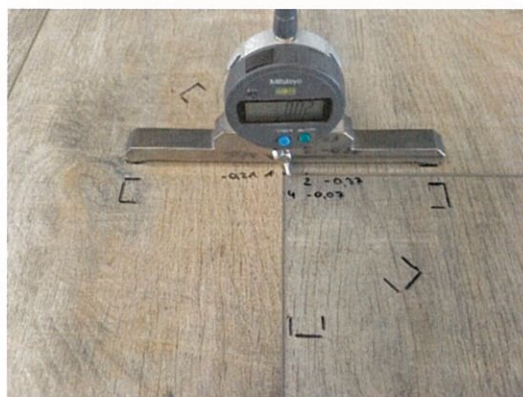
Figure 5: Example showing the markings for the supporting feet of the measuring device
